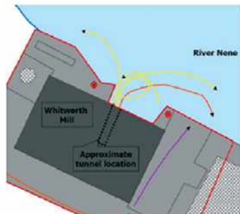
Plan 1 (Top left): Lighting design plan with bat flight paths marked Plan 2 (Top right): Site Plan including flight paths of bats over the River Nene Photo 1 (Bottom left): Bespoke lighting design solution
